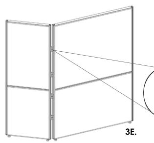
1. Once you attach the hinges on one panel, be sure to attach the hinges the opposite way on the second panel so one is angled north and the other is angled south(**3D**). The panels attach to each other by inserting one hinge into the other(see figure **3F**.). Lift Panel up slightly to insert hinges and connect the panels.
