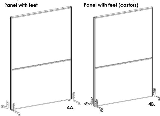
\*Note: If attaching 2 or more panels together use only one foot between two panels. (see below).
